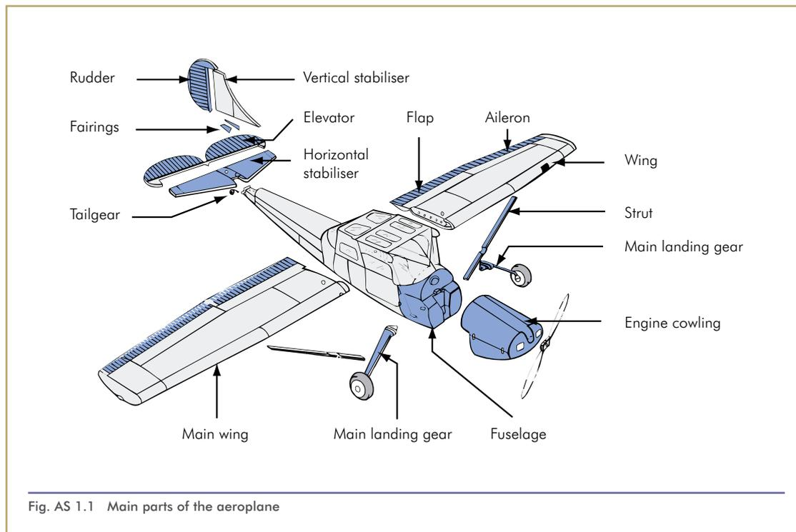
Fig. AS 1.1 Main parts of the aeroplane
